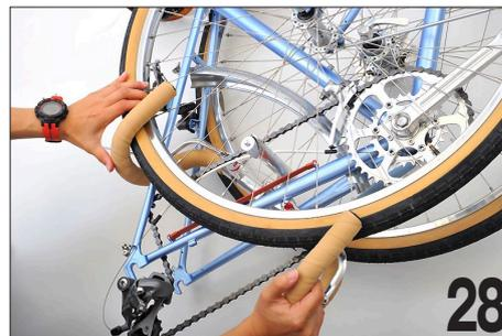
Slip the handle bars inside the rear triangle. Correct positioning uses the front tire to prevent the chain from touching the bar tape.
