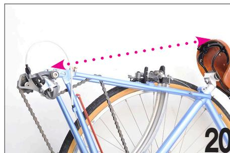
Imagine a line from the rear derailleur to the back of the saddle. This will be the plane (ground plane) that the bike rests on once it is properly bundled. Nothing should extend beyond it.
