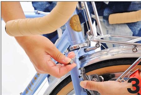
Unhook the straddle cable from the brake arm. Some brakes allow this on both arms. Others have the straddle bolted to the other arm.
