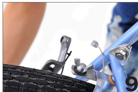
If your straddle wire is still attached to one side of your brakes, unhook the yoke from the straddle wire.
