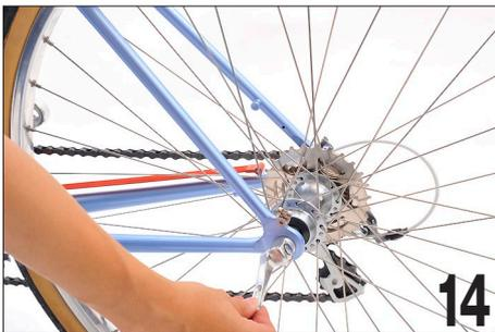
Open the rear quick release by moving the lever from the "close" position to the "open" position, as shown on the lever. It is not necessary to adjust the nut on the side opposite the lever.
