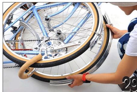
Place the rear fender around the rear wheel. Push the fender struts through the spokes to keep them from scratching anything and also to make the fender stay snug around the tire.
