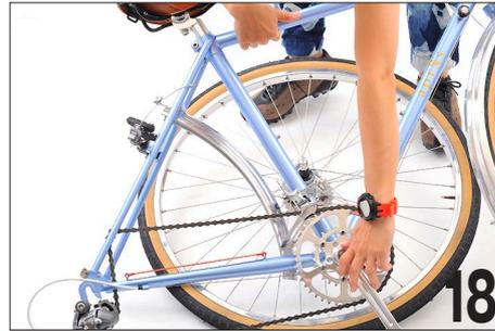
Lay the frame down on top of the rear wheel as shown. Note that the cassette/freehub is facing the ground.
