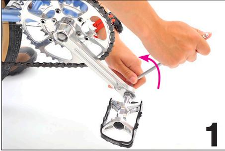
Unscrew the driveside pedal with the appropriate wrench, either a 6mm or 8mm Allen wrench or a 15mm open end depending on which type of pedal is on your bike.
