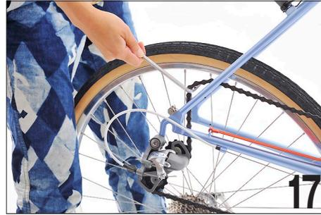
Use an allen key to place the chain on the chain rest on the inside of the seat stay. This will help keep your hands clean.
