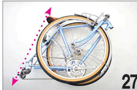
Note the alignment of the fork and front rack with the frame.
