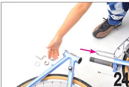
Remove all of the headset parts including the cable hanger from the steer tube (fork).
