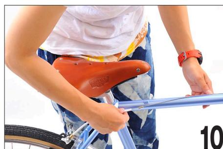
The stops are slotted to allow the inner wire to come free.
