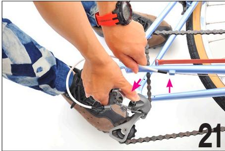
With the shifter in the highest gear (most difficult to pedal) push the derailleur towards the center of the bike. While holding it in this position remove the cable housing from the stop.
