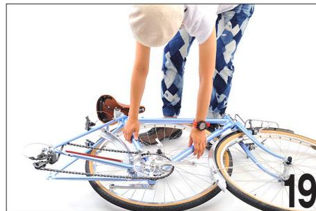
Arrange the frame carefully to avoid scratching. Use frame covers if needed.
