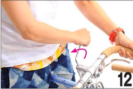
Loosen the stem bolt with a 6mm allen wrench. Only loosen it between a half and full turn (180-360 degrees).
