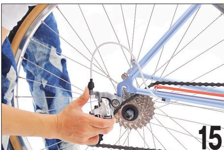
Pull the derailleur rearward to allow the wheel to drop free from the rear end.
