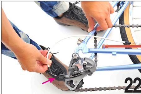
The rear derailleur housing is slid away from the derailleur. This allows the bundle to rest on the ground plane without damaging the derailleur, or affecting its adjustment. Refer to the picture on the cover if this is unclear.
